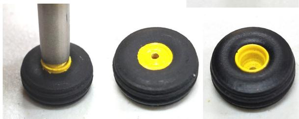
The flat side of the 17/64 drill bit works well for a press as it is the same diameter as the rim.
