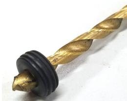
After painting the rims, use a 1/16" drill bit to ream the axle bearing of the rim. This will allow easier mounting to the axle and help prevent damage to the rim or axle mount.
